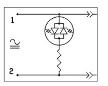
Status indicator (LED) and protective circuit (varistor)
